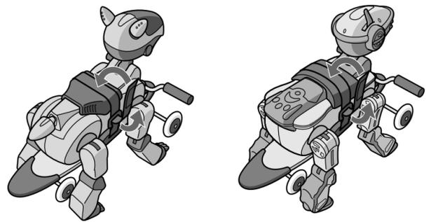
Secure AIBO to the Speed Board with its all legs stretched down
