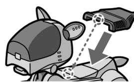
Line up the edge of the adapter with the line on AIBO's back.
