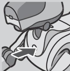
To turn AIBO off, press the Pause button located on its chest. Place AIBO in this mode before changing or replacing the battery or "Memory Stick."
