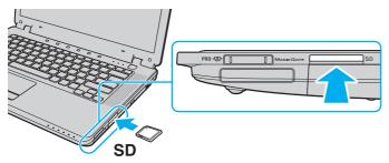
**3** Carefully slide the memory card into the slot until it clicks into place. Do not force the card into the slot.
