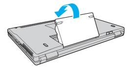
5 Slide the battery LOCK/UNLOCK switch to the LOCK position to secure the battery pack to the computer.
