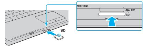
3 Carefully slide the memory card into the slot until it clicks into place. Do not force the card into the slot.
