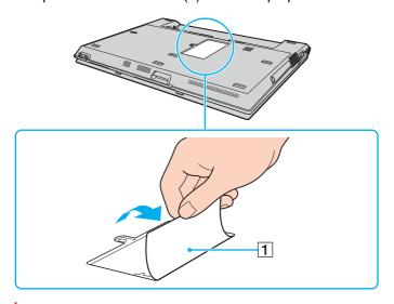
The insulation sheet is equipped for module protection. Do not pull it too hard to damage the sheet.
