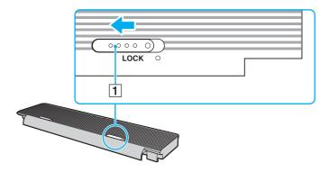
**3** Fit the battery pack into the battery compartment. The battery pack should be level with the bottom of the computer.
