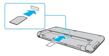
Do not touch the printed circuit on the SIM card. Be sure to hold your computer firmly before inserting or removing the card.
