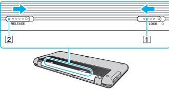
4 Lift the back-side edge of the battery pack to take it out of the battery compartment.
