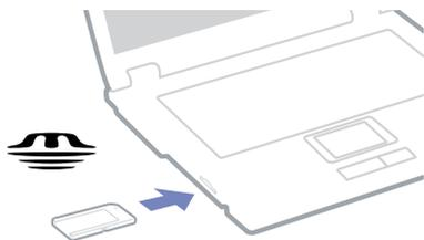
**!** Hold the Memory Stick with the arrow pointing in the correct direction when you insert it into the slot. To avoid damaging the computer or the Memory Stick, do not force the Memory Stick into the slot if it does not insert smoothly.
