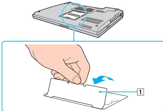
**!** The inflation sheet is equipped for module protection. Do not pull it too hard to damage the sheet.
