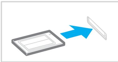
! Insert the PC Card slot protector to protect against debris entering the slot when not using a PC Card. Before carrying the computer, make sure to insert the PC Card slot protector into the slot.
