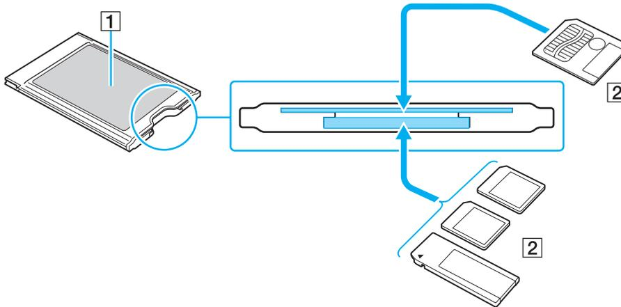
**!** Make sure to insert a memory card into the memory card adapter in the correct direction to avoid possible damage to the memory card adapter.
