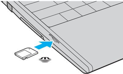
! Be sure to hold the Memory Stick media with the arrow pointing in the correct direction as you insert it into the slot. To avoid damaging the computer or the Memory Stick media, do not force the Memory Stick media into the slot if it does not insert smoothly.
