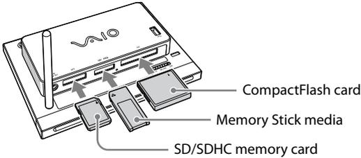
When removing Memory Stick, Memory Stick PRO, Memory Stick Duo or Memory Stick PRO Duo media, or an SD/SDHC memory card, make sure the media access indicator is not lit. Push fully in once and pull out. When removing a CompactFlash card, make sure the media access indicator is not lit.
