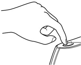
Press and hold the AOSS button until the access point indicator blinks.
