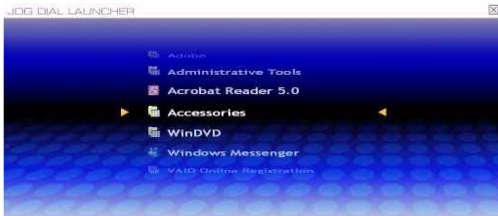
Rotate the Jog Dial™ up and down to view the software applications and utilities on your computer. To launch an application, make sure it is selected and press the Jog Dial™.
