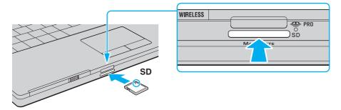
3 Carefully slide the memory card into the slot until it clicks into place. Do not force the card into the slot.
