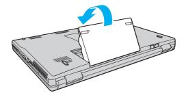
5 Slide the battery LOCK/UNLOCK switch to the LOCK position to secure the battery pack on the computer.
