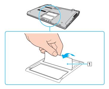
! The insulation sheet is equipped for module protection. Do not pull it so hard as to damage the sheet.
