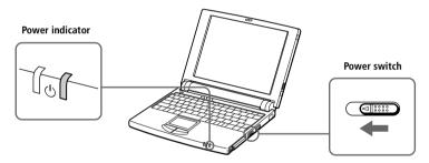
A If you hold the power switch in the on position for more than four seconds, the computer turns off.
