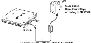
AC adapter cable (SELV, according to EN 60950)
