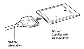
4 Insert the PC card into the PC card slot with the label side facing up. See "Using PC Cards" on page 26 for details.
