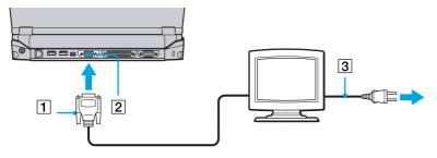
If the main unit is docked, you can only use the monitor connector on the docking station
