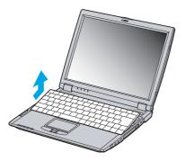
Lift the keyboard from the LCD display side, then gently turn it over the touchpad. Be careful not to detach the cable (1) when lifting the keyboard.
