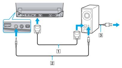
If the main unit is docked, you can only use the monitor connector on the docking station.
