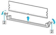
6 Grasp the memory module by the sides and remove from the main unit. Store the module in a static-free bag.
