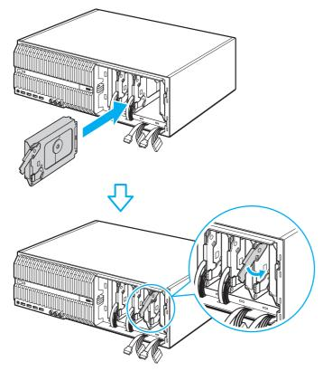
Connect the power connectors to the preinstalled and new hard disk drives.
