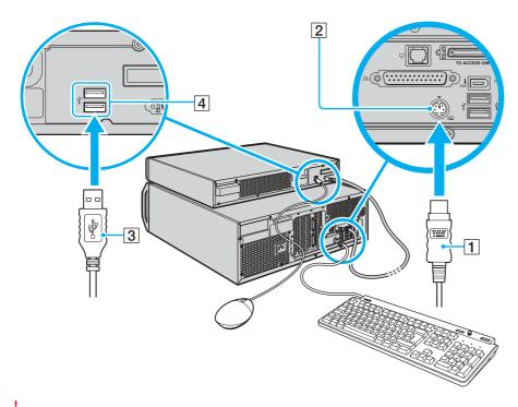
! Be sure not to connect the mouse to any USB port on the main unit. The mouse will not be functional.
