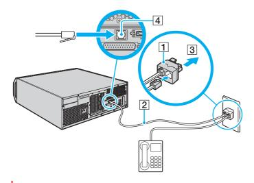
The main unit has a protective sticker covering the network (Ethernet) port located on its back. Connect 10BASE-T, 100BASE-TX, or 1000BASE-T cable to the network (Ethernet) port. Using an incorrect cable, such as a phone cable, may result in an electric current overload that can cause a malfunction, excessive heat, or fire in the network (Ethernet) port. For help on connecting to a network, see your network administrator.
