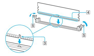
To avoid damaging a memory module or the memory module slot, move the side latches slightly outward to relieve pressure.
