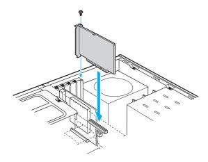
Be careful not to touch other internal components when inserting the card as it may cause a failure.
