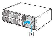
2 Insert the tabs (2) on the right edge of the plastic HDD cover underneath the chassis frame and push in the left end of the cover.
