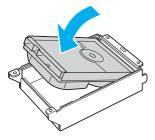
6 Replace the holder cover and secure it with the screws.
