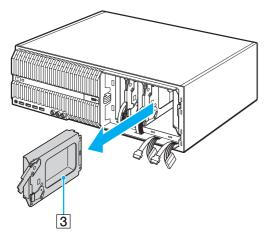
4 Unscrew the four screws from the holder cover.
