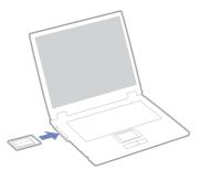
Gently push the PC Card slot into the connector.
