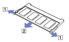
7 Pull the memory module in the direction of arrow 2.
