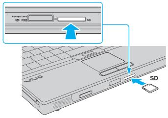
3 Carefully slide the memory card into the slot until it clicks into place. Do not force the card into the slot.
