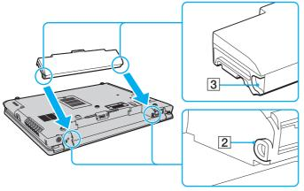
4 Rotate the battery pack in the direction of the arrow, and push the battery pack down into the compartment until it clicks into place.
