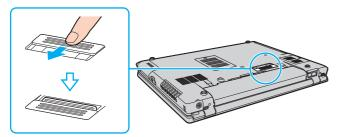
5 Slide the **LOCK/UNLOCK** switch on the multi function bay docking station to the **UNLOCK** position.
