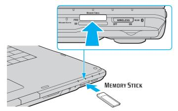
Be sure to hold the Memory Stick media with the arrow pointing in the correct direction as you insert it into the slot. To avoid damaging your computer or the Memory Stick media, do not force the Memory Stick media into the slot if you cannot insert it smoothly.
