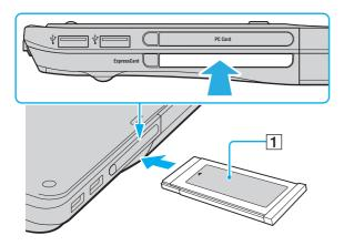
insert the ExpressCard slot protector to protect against debris entering the slot when not using an ExpressCard module. Before moving your computer, be sure to insert the ExpressCard slot protector into the slot.
