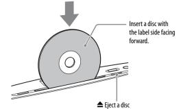
Playback starts automatically after "READING" disappear
