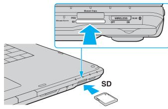
**3** Carefully slide the memory card into the slot until it clicks into place. Do not force the card into the slot.
