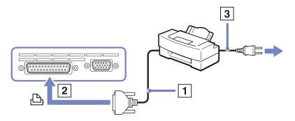
/ Turn off your computer and the printer, unplug the AC adapter and the power cord before connecting the printer.
