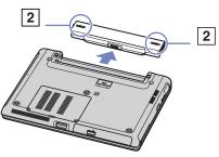
🆄 You can remove the battery pack without turning off the computer if it is connected to the mains voltage (AC adapter).
