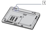
3 Slide and hold the release lever (2) as indicated and slide the battery away from the computer.
