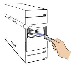
Make sure the memory stick is secure in the slot. The memory stick is automatically detected by your system and appears in the **My Computer** window with its own drive.
