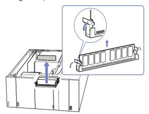
6 To insert a new memory module, remove it from its anti-static package, handling it only by the edges.
