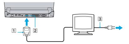
$\swarrow$  If the main unit is docked, you can only use the monitor connector on the docking station
