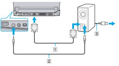
$\swarrow$  If the main unit is docked, you can only use the monitor connector on the docking station.
