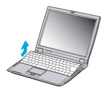
7 Lift the keyboard from the LCD display side, then gently turn it over the touchpad. Be careful not to detach the cable (1) when lifting the keyboard.
