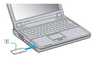
Hold the Memory Stick<sup>TM</sup> with the arrow pointing in the correct direction when you insert it into the slot. To avoid damaging the computer or the Memory Stick<sup>TM</sup>, do not force the Memory Stick<sup>TM</sup> into the slot if it does not insert smoothly.
