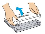
Do not undock the notebook when the docking station indicator is on. If you undock when the docking station indicator on the notebook is on, you may lose data or malfunction may occur. Make sure all cables and peripherals are removed before disconnecting the main unit from the docking station.
