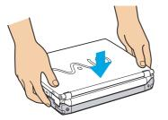
$\swarrow$  You cannot connect the docking station when the notebook is in a power saving mode. Return to normal mode before docking.
