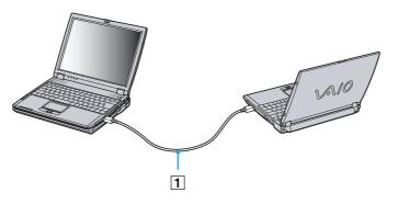
If the notebook is connected to the optional docking station, proceed as follows to exchange data with another computer using an i.LINK<sup>™</sup> cable (also optional):
