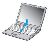
12 Close the computer cover, then tighten the screws on the bottom of the computer.
