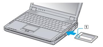
2 Gently push the card into the slot until the card is fixed into the connector.
