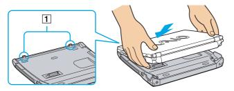
5 Press the bottom of the notebook on the docking station until you hear two clicks. The docking station is now connected to the computer.
