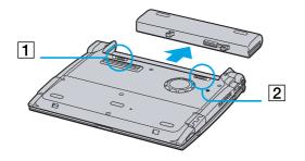
Kou can remove the battery pack without turning off the computer when it is connected to the mains voltage (AC adapter).
