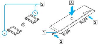
If any key top other than the above keys falls off, see the figure below to place it back into position.
