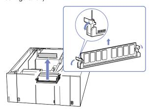
6 To insert a new memory module, remove it from its anti-static package, handling it only by the edges.
