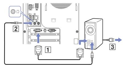
This illustration may not correspond to the configuration of your model. Please check the section **Back Panel** of your printed **Specifications** sheet to see where the ports are exactly.
