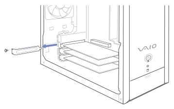
Install the add-on board by sliding it into the expansion slot and secure it with the screw from the expansion slot cover, as shown (may vary from actual configuration):
