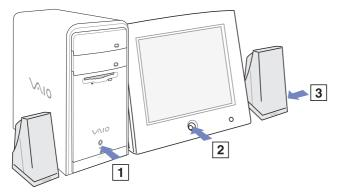
if you press the computer's power button for more than six seconds, the system will switch itself off.
