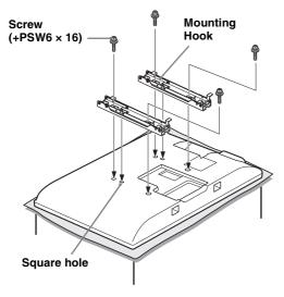
Align the tab on the rear of the Mounting Hook with the square hole on the rear of the TV as in the illustration below.
