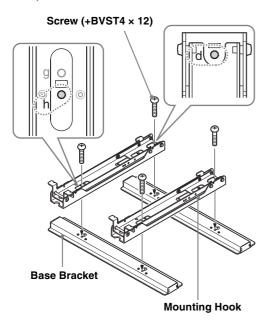
2 Secure the Base Bracket and the Mounting Hook on the wall using the four or more 8 mm diameter or equivalent screws (not supplied).
