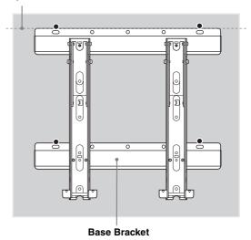
**3** Remove the screws which were attached in procedure **1** and detach the Mounting Hook from the Base Bracket.
