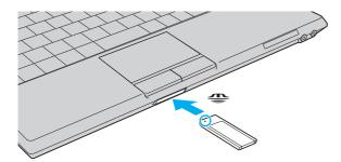
Be sure to hold the Memory Stick media with the arrow pointing in the correct direction as you insert it into the slot. To avoid damaging your computer or the Memory Stick media, do not force the Memory Stick media into the slot if you cannot insert it smoothly.
