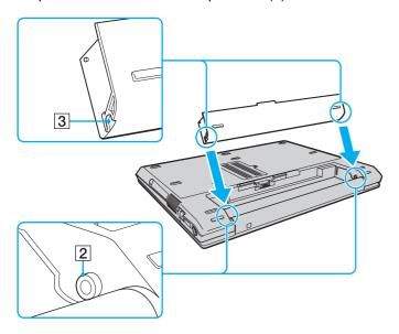
4 Rotate the battery pack in the direction of the arrow, and push the battery pack down into the compartment until it clicks into place.
