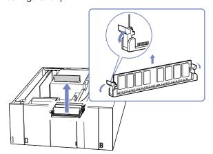
6 To insert a new memory module, remove it from its anti-static package, handling it only by the edges.
