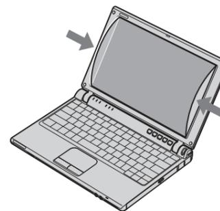
Insert your fingernails in the spaces at the left and right edges of the Privacy Filter, and remove it carefully as illustrated.
