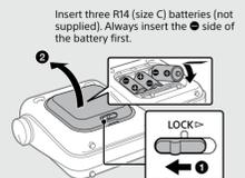
Insert three R14 (size C) batteries (not supplied). Always insert the (+) side of the battery first.
